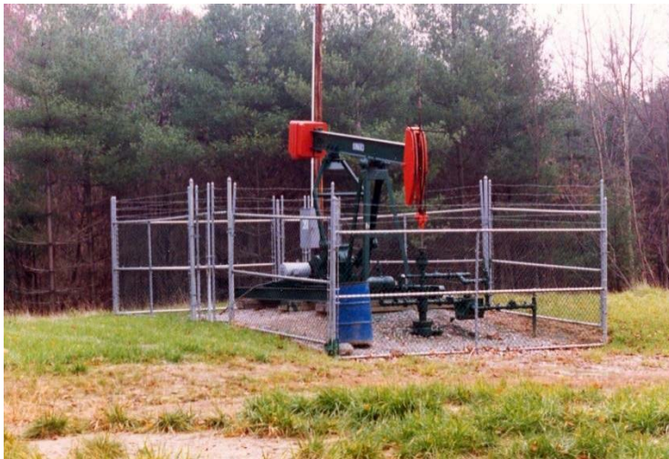
Oil well at Cuyahoga Valley National Park, Ohio. This is an example of a well maintained oil well with proper fencing, signage, and good site maintenance. (NPS photo)
