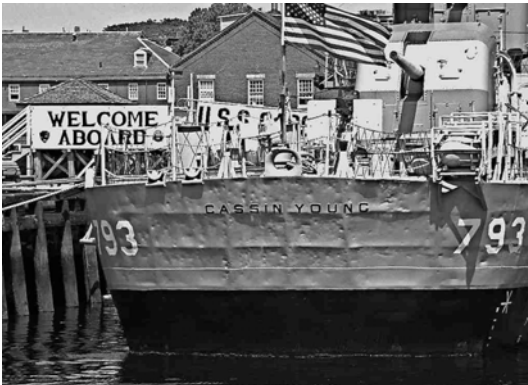
The Cassin Young stern (left) and hull (right). The frame of the ship is visible through the thin quarter inch steel hull. There is a 70% loss of the original hull thickness (one-quarter inch) in some places.
