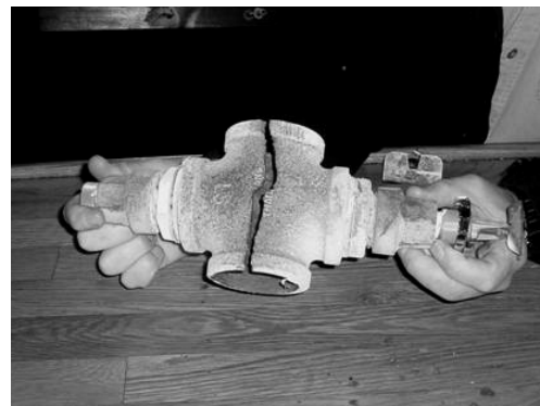
A cracked fire suppression valve, which has been replaced, reflects the current condition of similar component deterioration.
