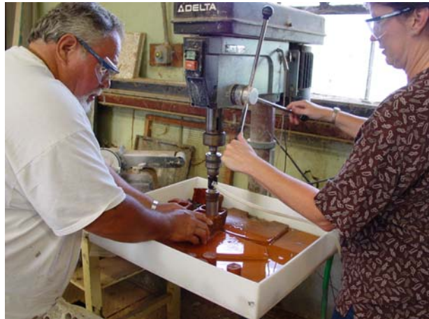
Using coring equipment to create samples for National Center for Preservation and Technology research on limewash recipes held at Cane River Creole NHP.
